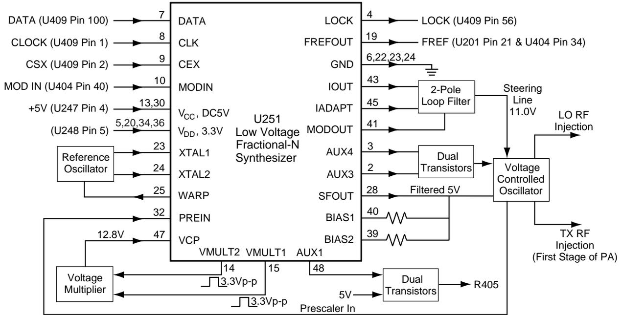
Figure 2-27. Synthesizer Block Diagram
