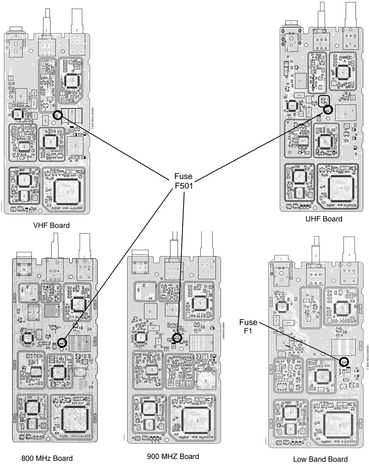
Figure 3-1. UHF/VHF/Low Band/800 MHz/900 MHz Circuit Board Fuse Locations
