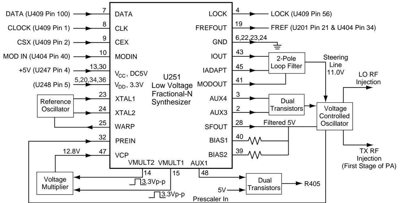
Figure 2-22. 800 MHz Synthesizer Block Diagram
