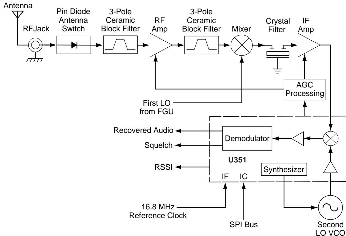
Figure 2-25. 900 MHz Receiver Block Diagram
