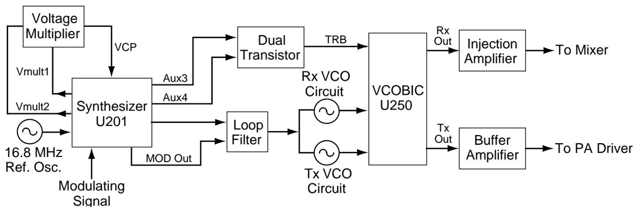
Figure 2-26. Frequency Generation Unit Block Diagram
