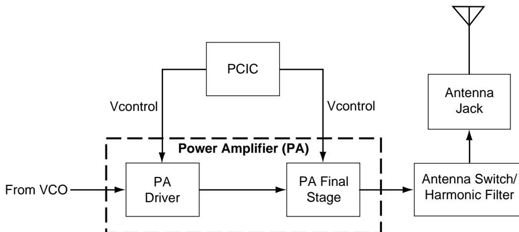
Figure 2-24. Transmitter Block Diagram
