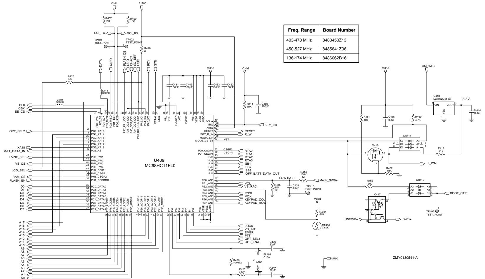
Figure 4-13: VHF/UHF Controller Micro Processor Schematic Diagram
