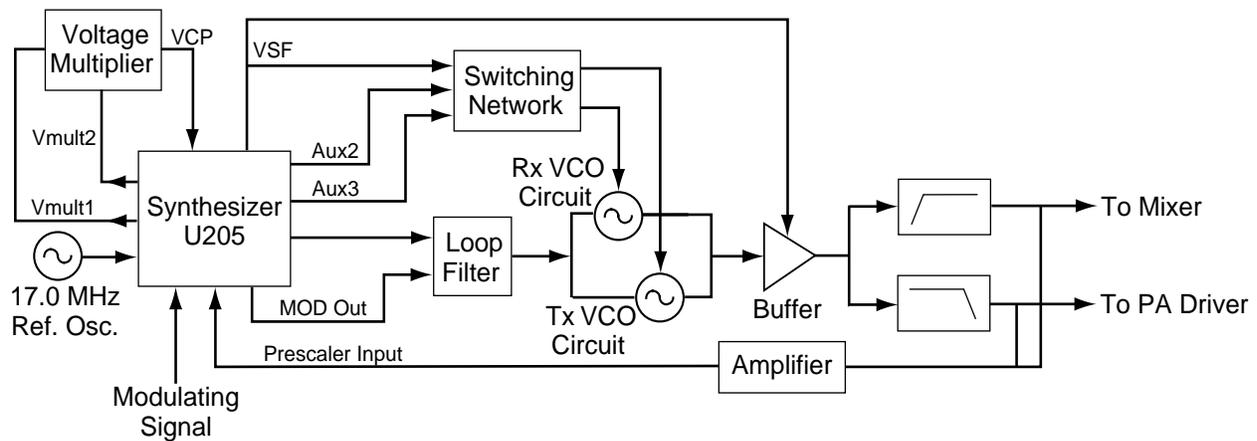
Figure 2-17. Low Band Frequency Generation Unit Block Diagram
