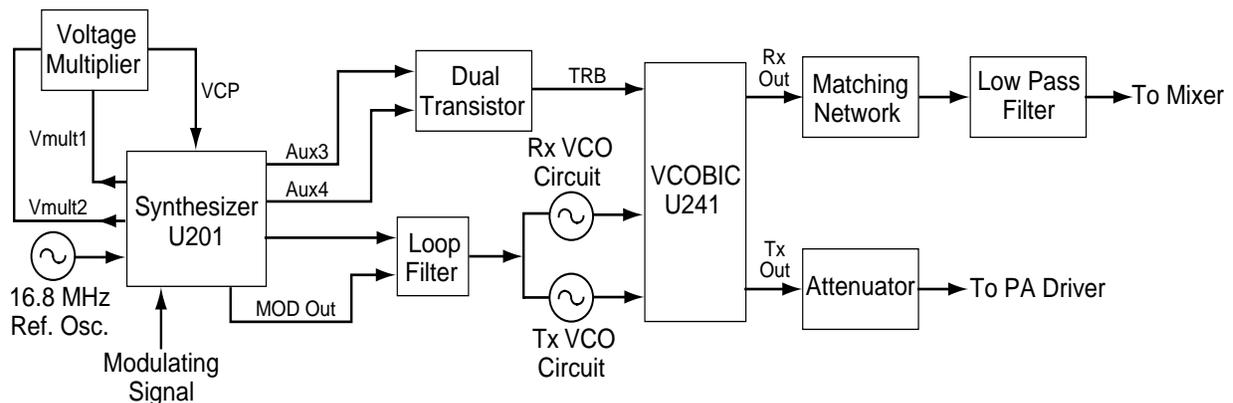
Figure 2-7. UHF Frequency Generation Unit Block Diagram
