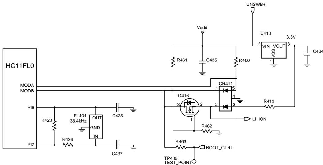
Figure 2-4. RTC Circuit
