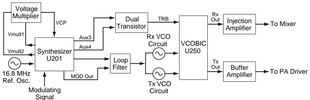
Figure 2-21. 800 MHz Frequency Generation Unit Block Diagram
