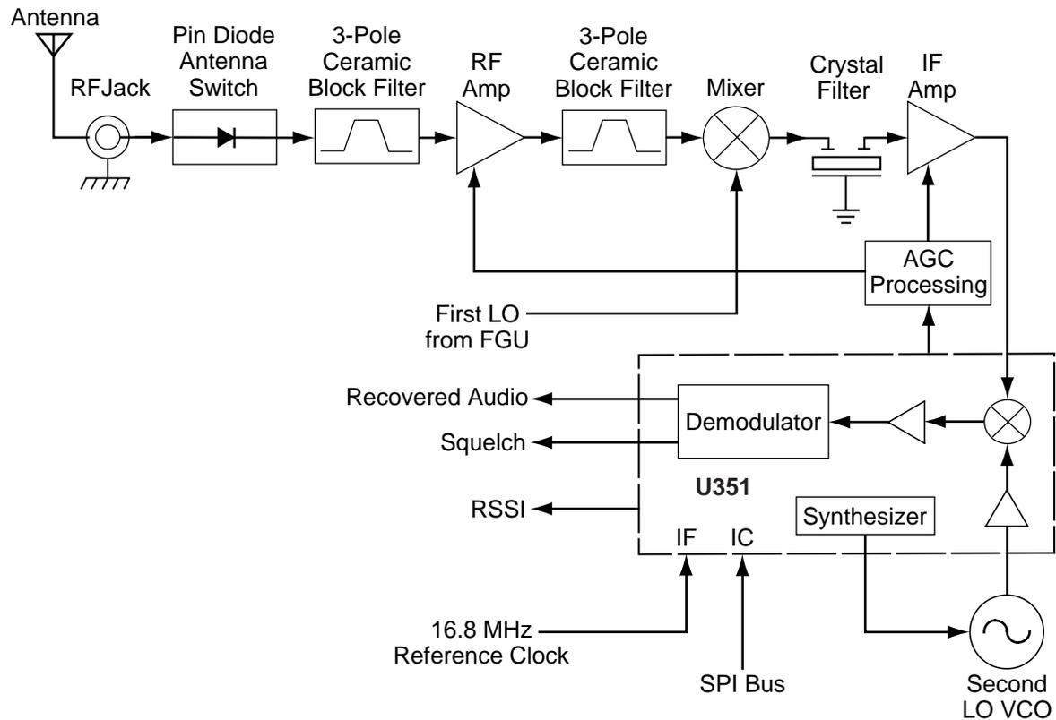
Figure 2-20. 800 MHz Receiver Block Diagram
