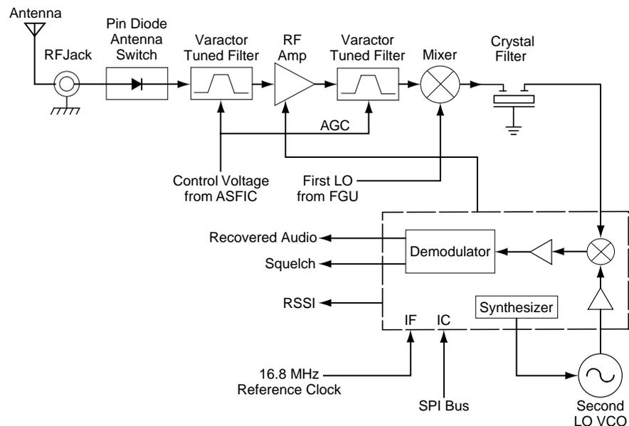
Figure 2-11. VHF Receiver Block Diagram
