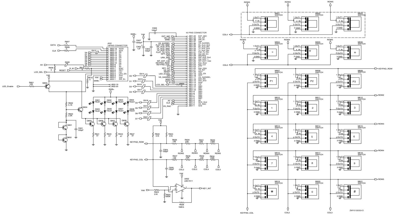
Figure 4-8: 9000 Series Keypad Board Schematic Diagram
