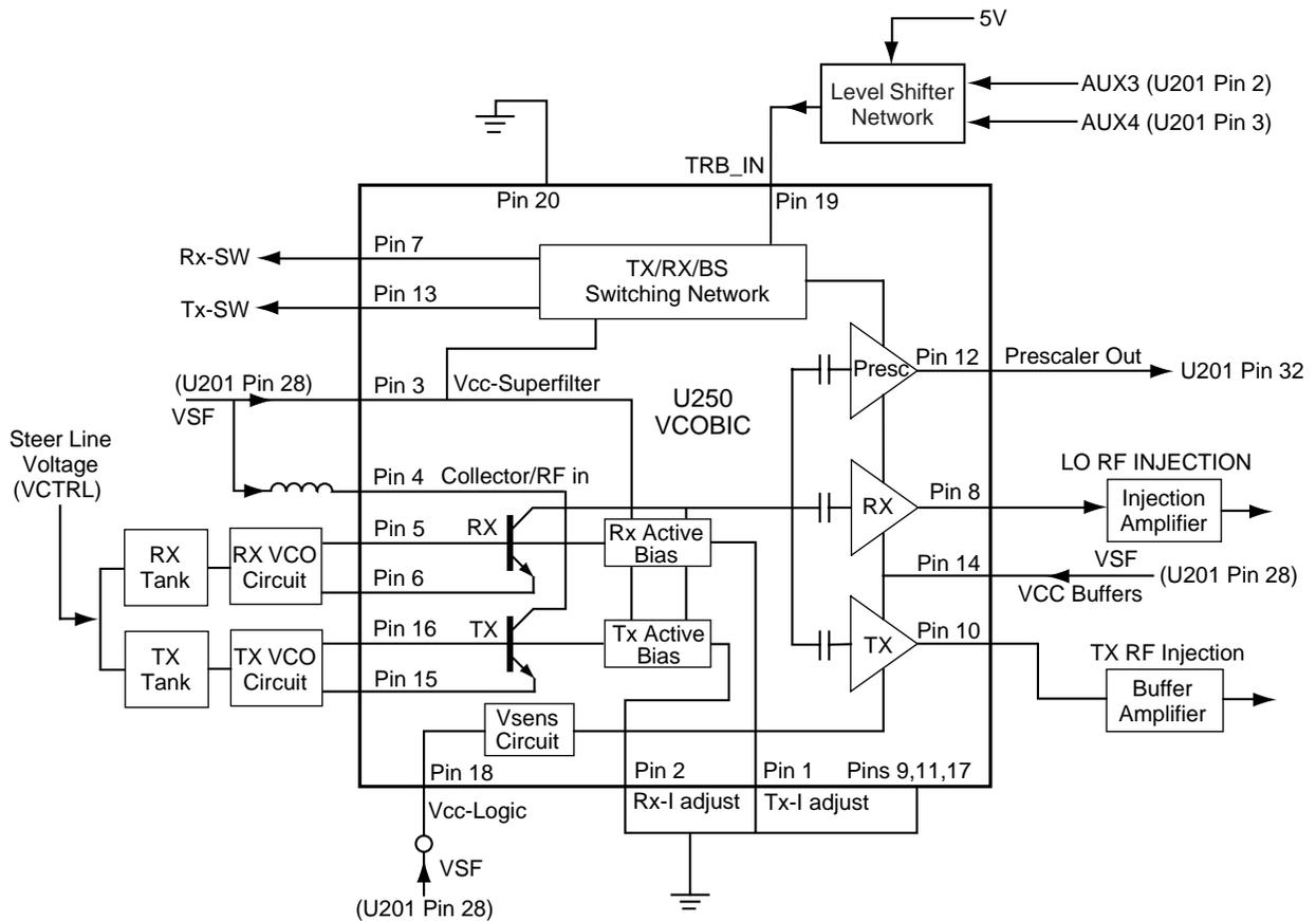
Figure 2-28. VCO Block Diagram
