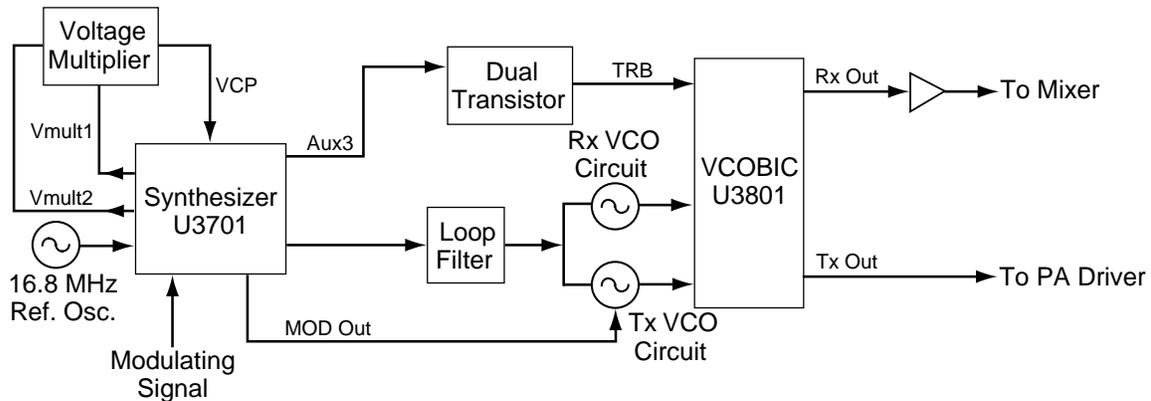
Figure 2-12. VHF Frequency Generation Unit Block Diagram
